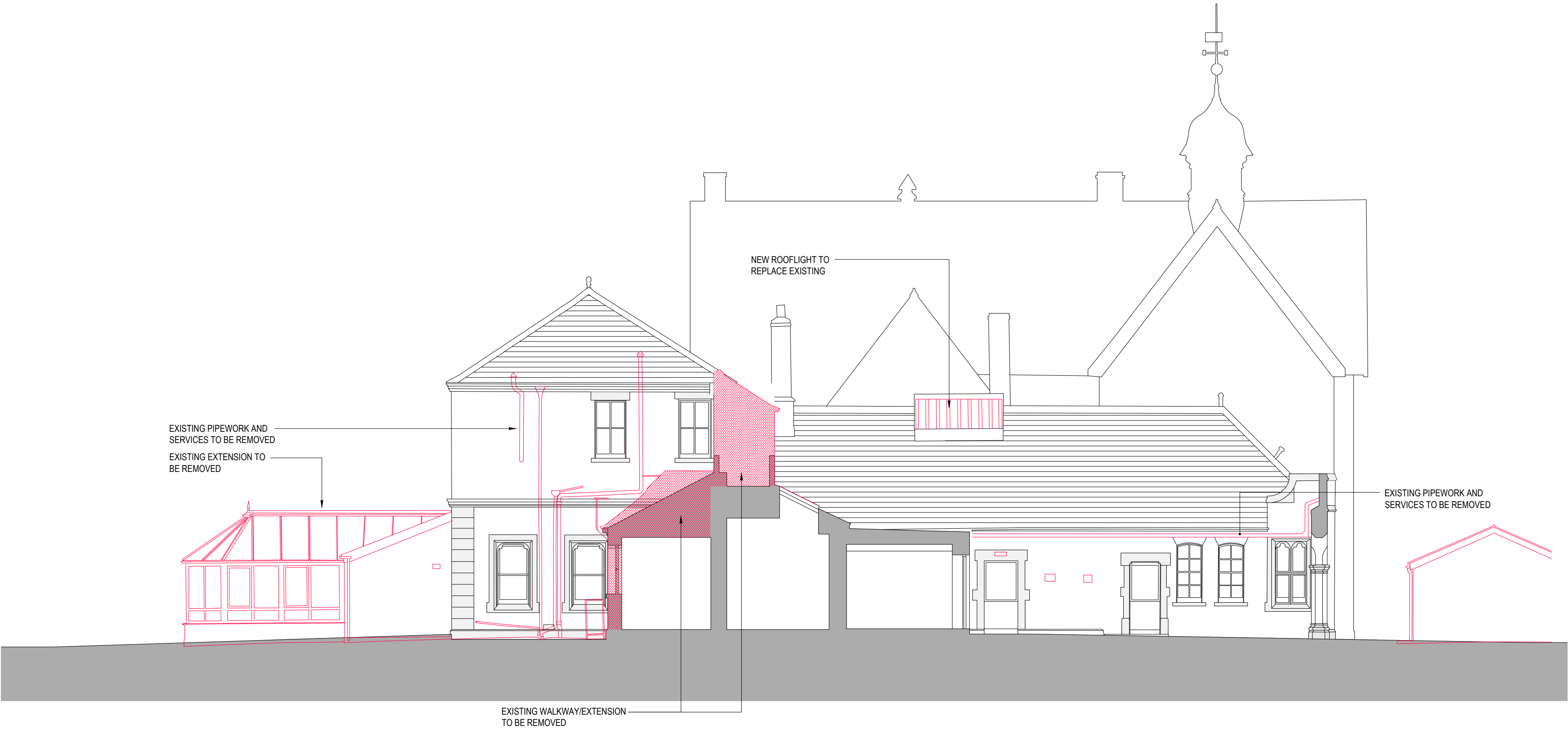
ELEVATION 06 - REMOVALS SCALE 1:100
