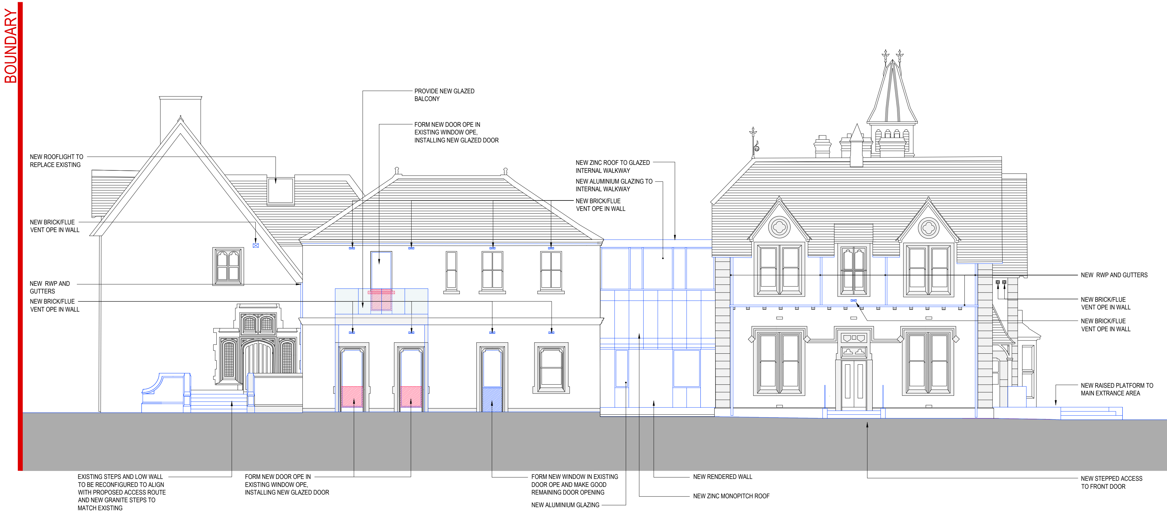
ELEVATION 02 - SOUTH EAST - ADDITIONS SCALE 1:100
