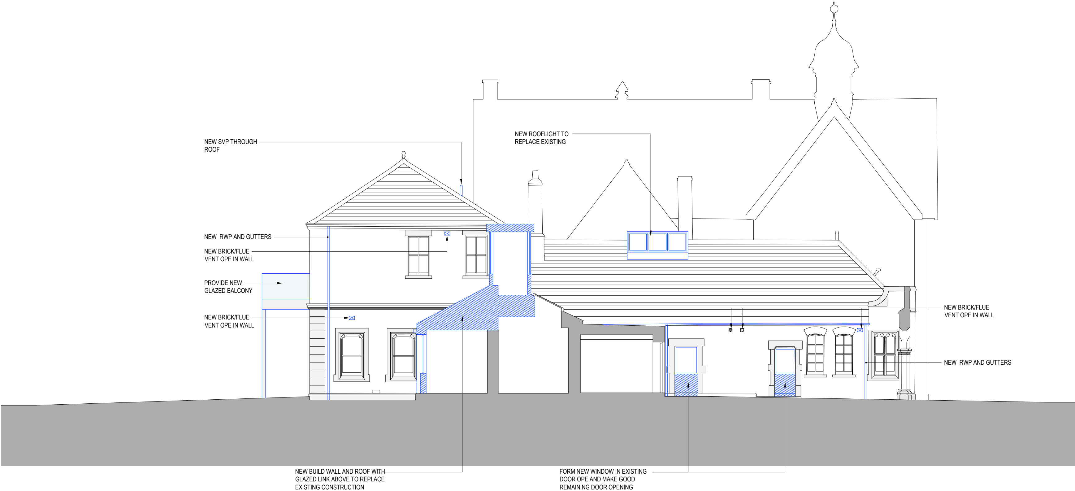
ELEVATION 06 - ADDITIONS SCALE 1:100
