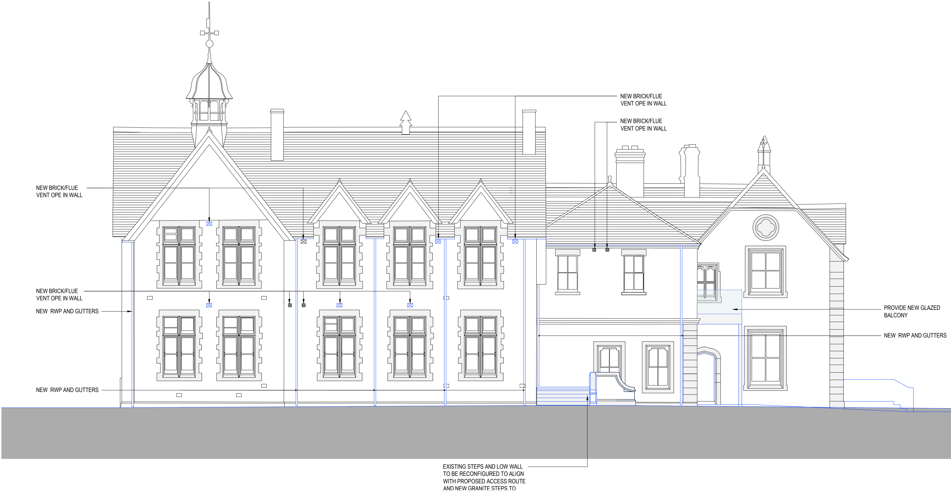
ELEVATION 01 - SOUTH WEST - ADDITIONS SCALE 1:100
