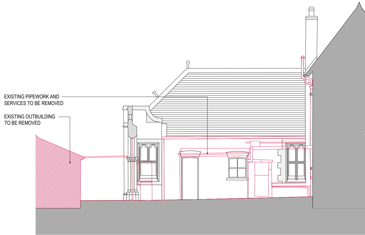
ELEVATION 07 - REMOVALS SCALE 1:100
