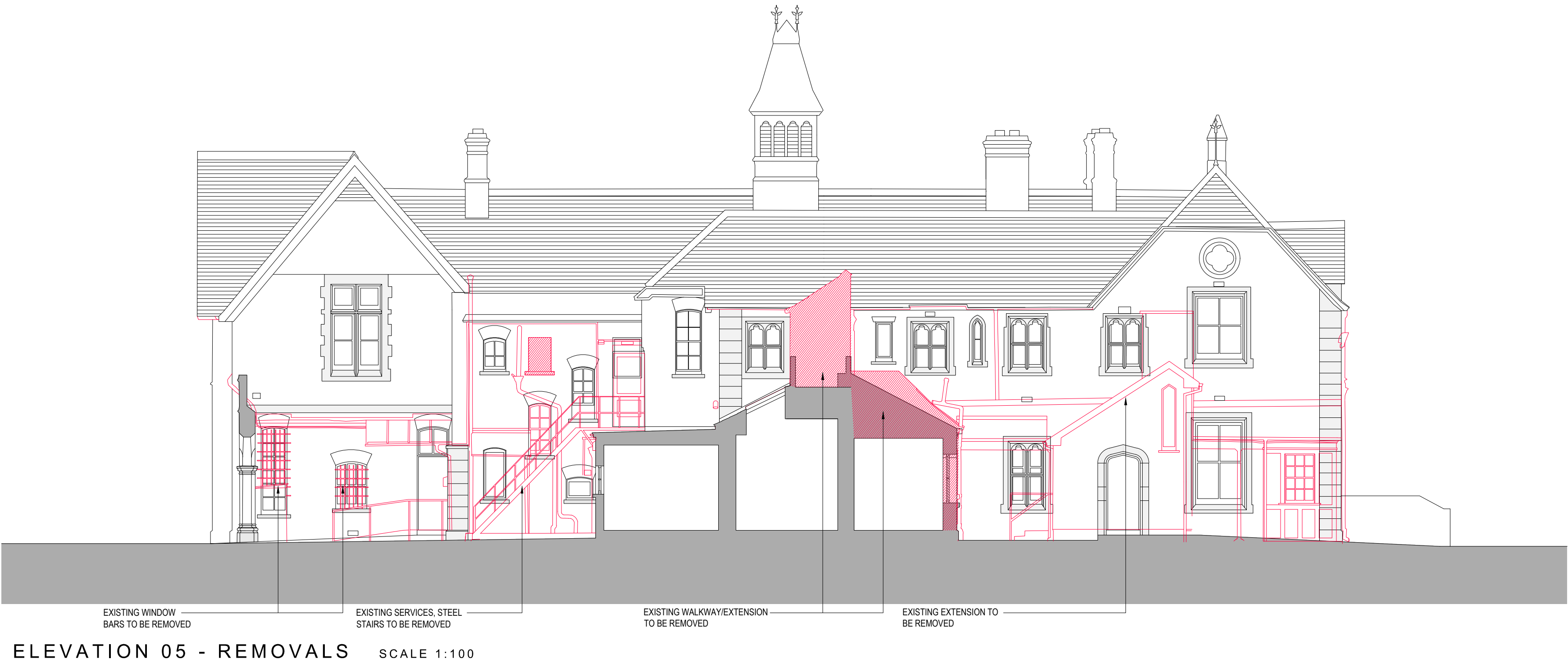
ELEVATION 05 - REMOVALS SCALE 1:100
